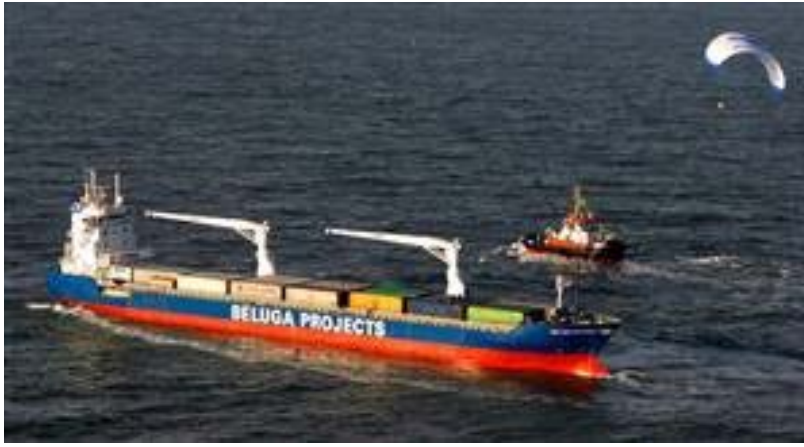
The 'Beluga SkySails' is seen Tuesday with its kite helping pull it along
